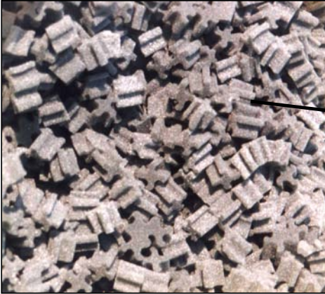
PU foam Carriers – Highly porous for microorganism growth
